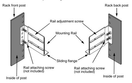
Figure 2. Mounting rail installation
